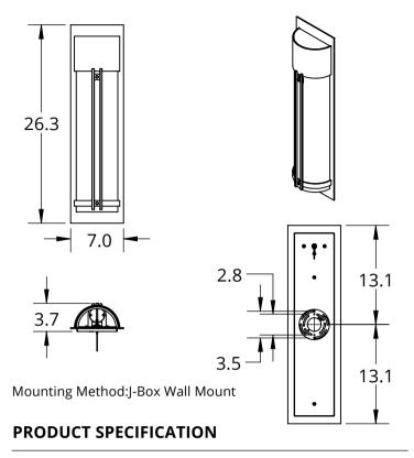
Construction: Aluminum Body With Formed Glass
