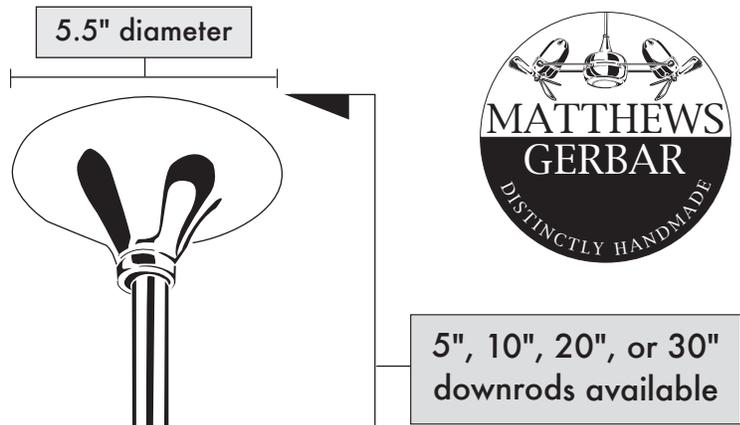
Fan head is infinitely adjustable 180° in forward and reverse positions.
