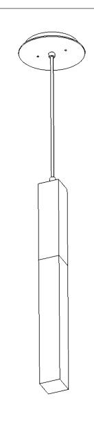
\*\* NOTE\*\* DRIVER TO BE INSTALLED IN J-BOX. MINIMUM SIZE OF J-BOX REQUIRED IS 4" L x 4" W x 1.5" H
