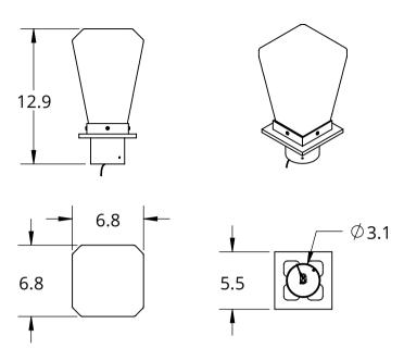
Mounting Method: Mounts Directly To Post
