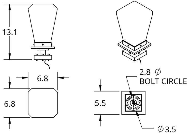
Mounting Method:Mounts Directly to Pier
