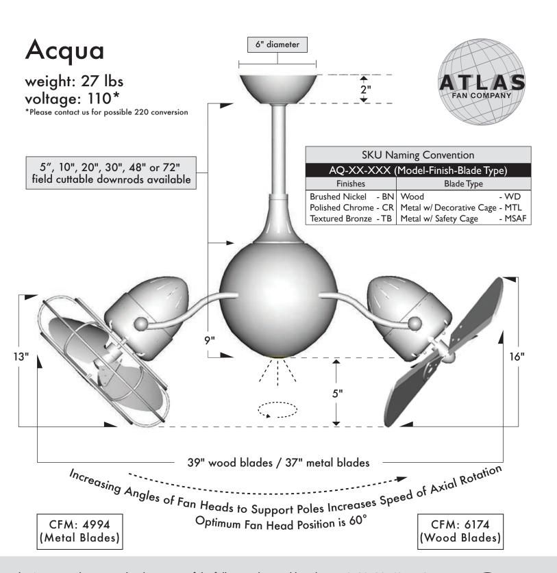
The Acqua can be mounted with any one of the following downrod lengths: 5, 10, 20, 30, 48 or 72".
